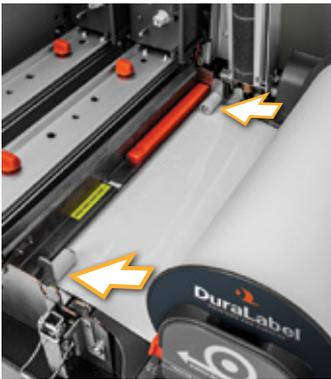
4. Slide the adjustable supply guides together ensuring the supply remains between the two guides and under the white rollers. Push the supply forward, under the metal guide with the orange sensor to the line shown on the yellow label.
