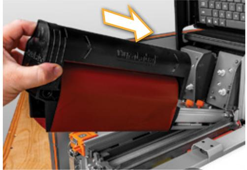
2. Holding the ribbon cartridge on the side imprint with the DuraLabel logo (with the rolls facing up), insert it into the printer so the loose section of ribbon, on the bottom side of the ribbon cartridge, is positioned beneath the print head.
